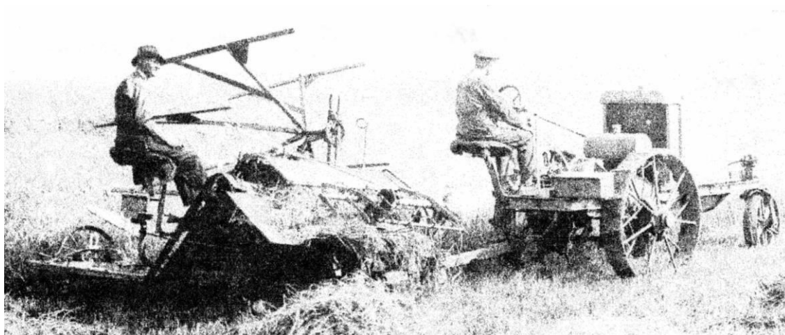
The Crawley Agrimotor hauling a reaper-binder harvesting at Howe Hall, Littlebury Green in the 1920s. Ernie Morris on the tractor and Charles Casbolt on the binder. Photograph © Nick Crawley.
